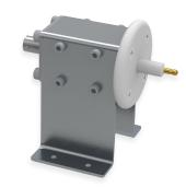
The RFP250 series high voltage probes are capacitive dividers designed to cover the 25 MHz to 250 MHz frequency range and voltages of up to 10 kV RMS. The output impedance is 50  $\Omega$  and they are very compact allowing mounting in tight spaces.
