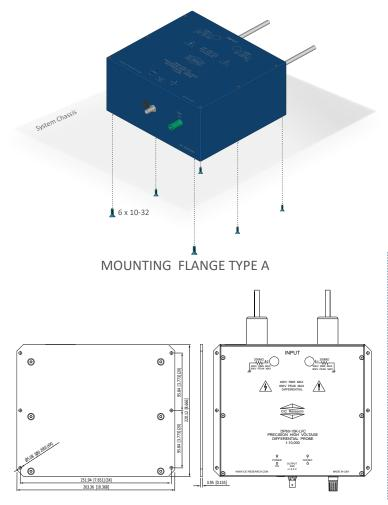
DP60 series probes can be mounted directly on a base plate or enclosure walls with 6 x 10-32 screws.
